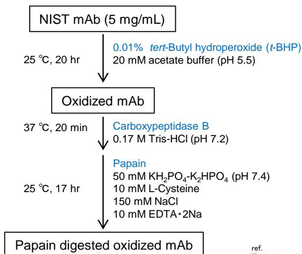
*tert*-Butyl hydroperoxide (*t*-BHP) was used as a chemical oxidant to promote oxidation of methionine residues of NIST mAb. Subsequently, papain was used for the preparation of two Fab fragments and one Fc fragment.
