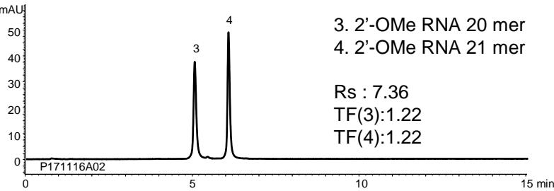
Good separation without carry-over and peak tailing of oligonucleotides was achieved by optimization of buffer/counter ion in the mobile phase and gradient profile, and by using BioPro IEX QF, non porous anion exchange column.
