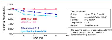
YMC-Triart C18, which offers excellent durability even under elevated temperature and low-pH conditions, is effective for the separation of peptides and proteins.
