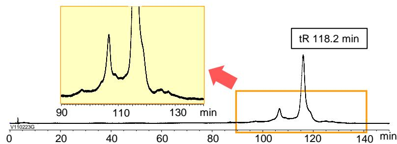
The separation of MAb is compared on SCX (BioPro IEX SF) and WCX (competitor's) under the same gradient condition at pH 5.6.
