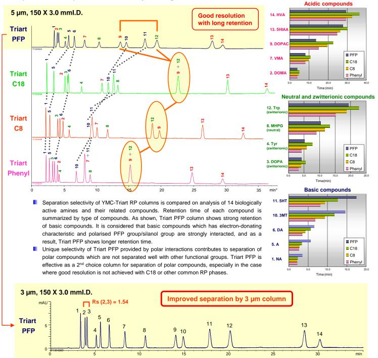
By changing the size from 5 µm to 3 µm, separation of DOMA (peak 2) and DOPA (peak 3) is improved.
