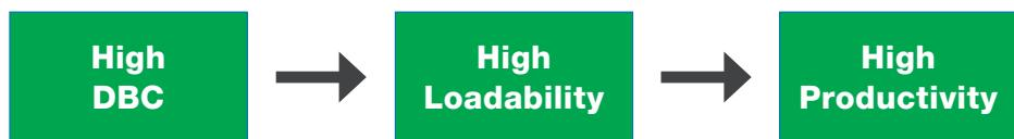
In contrast to the static binding capacity (SBC), where the maximum target binding of the bulk resin is measured, the DBC is a real process parameter as it is determined using the chromatographic setup. Therefore, modern process resins with maximum DBC are needed for increased productivity.
