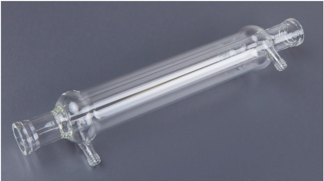
Borosilicate glass 3.3 heating jacket provides full organic solvent compatibility for efficient cleaning. This can drastically extend the column lifetime.
