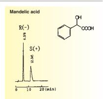
Column : SUMICHIRAL OA-6100 (150×4.6 mm) Mobile phase : 2 mmol/L copper(  ${\rm I\hspace{-.1em}I}$  ) sulfate in [water/
