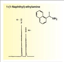
Column : SUMICHIRAL OA-8000 (250×4.6 mm) Mobile phase : perchloric acid in water (pH 2.0)/
