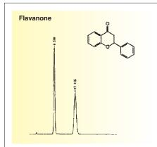
Column : SUMICHIRAL OA-7000 (250×4.6 mm) Mobile phase : 20 mmol/L phosphate buffer (pH 2.0)/
