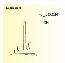
$\begin{array}{ll} \text{Column} & : \text{SUMICHIRAL OA-5000 (150} \times 4.6 \text{ mm}) \\ \text{Mobile phase : 2 mmol/L copper( $\mathbb{I}$ ) sulfate in [water/ $\mathbb{I}$ ) } \\ \end{array}$
