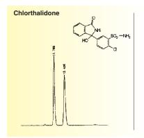
Column : SUMICHIRAL OA-7000 (250×4.6 mm) Mobile phase : 20 mmol/L phosphate buffer (pH 3.0)/
