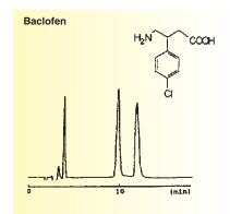
Column : SUMICHIRAL OA-5000 (150x4.6 mm) Mobile phase : 2 mmol/L copper( II ) sulfate in [water/
