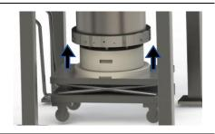
② Check that the seal is loose, and the end cap is lifted, and then loosen the clamp.
