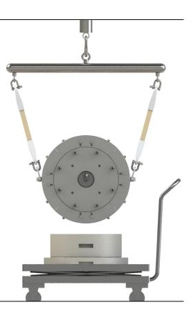
① Turn the end cap so that the filter surface is at the bottom while lifting.
