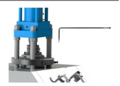
④ Operate the cylinder and lower it to the bottom and then put the lift table truck under the movable stopper. At this time, confirm that the top plate of the lift table truck is at the lowest position. (Turn the valve under the handle to the left to lower the table.)
