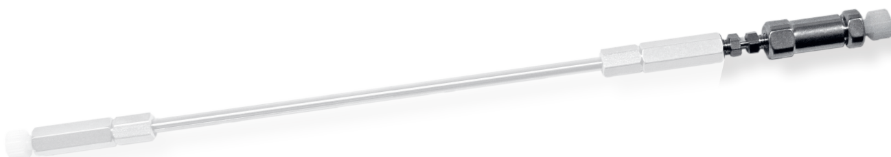
1/32" guard column coupled to a 1/32" analytical column.
