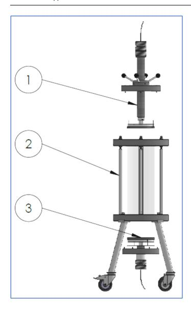
The glass column consists of the adjustable end piece (1), the column body (2), the fixed end piece (3) and the column stand. The column stand is fixed to the column body. The adjustable and the fixed end piece can be removed from the column body.
