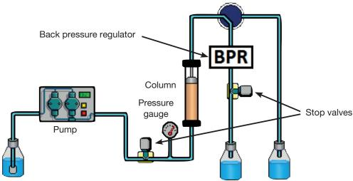
Fig. 3.2: Schematic overview of a system for a pressure test
