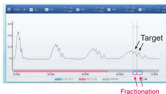
After the change of method parameters, you can check if the new fractionation window works.
