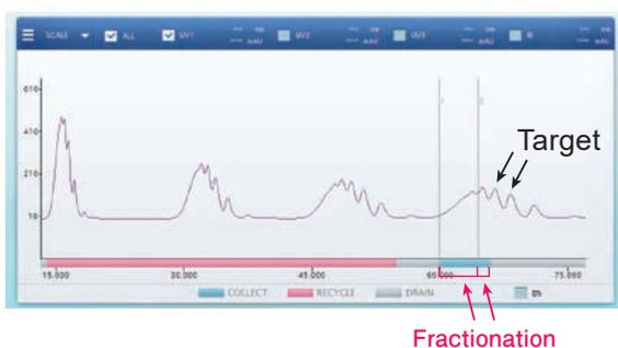
Preview Function enables to find and avoid error setting for fraction collection easily.
